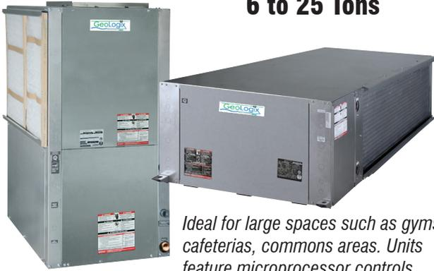
Ideal for large spaces such as gyms, cafeterias, commons areas. Units feature microprocessor controls, performance monitoring system and dual refrigerant circuits. Available in front or back return, and a variety of discharge locations and voltages. Cabinets are fully insulated and scroll compressors have special double isolation mounting system for quiet operation. **HB Large** capacity models available in horizontal and vertical configurations.
